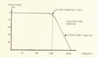
The vertical axis shows the amount of attenuation, while the horizontal axis gives the frequency. As you can see, a low-pass filter allows the lower portion of the frequency spectrum to pass without significant attenuation, but attenuates the upper portion. The frequency above which the amount of attenuation increases rapidly is called the cutoff frequency, while the characteristic rate at which the attenuation increases as the signal frequency goes above cutoff is called the cutoff slope.
